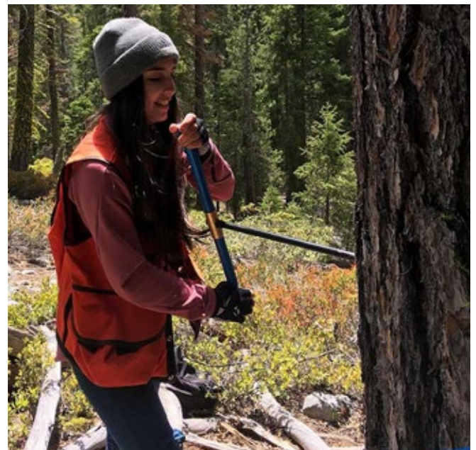
The team from Cal Poly Humboldt uses an increment borer to core a sugar pine.
